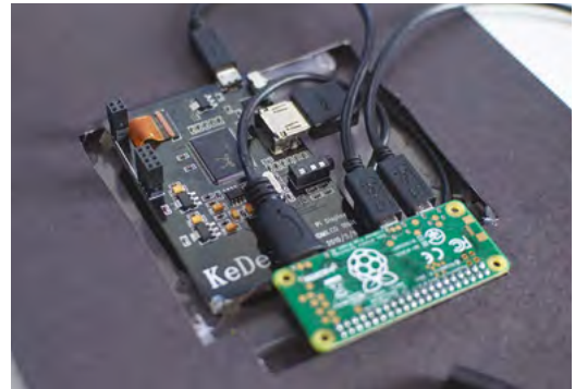
▲ As well as connecting via GPIO, Raspberry Pi Zero can be simply hooked up using cables
