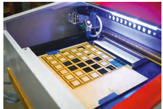
▲ Alex eventually got a laser cutter to help speed up production – like for these mounting grids
