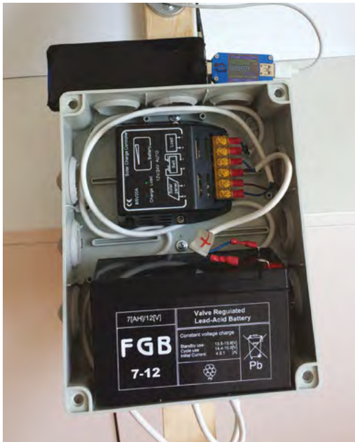
▲ A 12V, 7Ah lead-acid battery has been sufficient to provide an average power consumption of 2W since it can provide 84 watt-hours of energy
