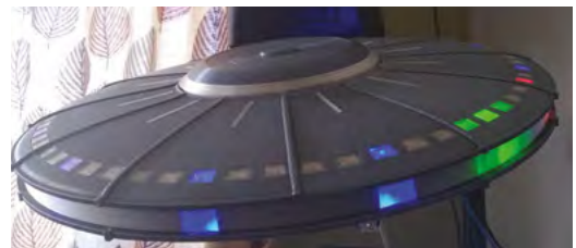
▲ A side view of the saucer. Transparent segments are used to diffuse the LEDs, with light blockers between them for crisp separation
