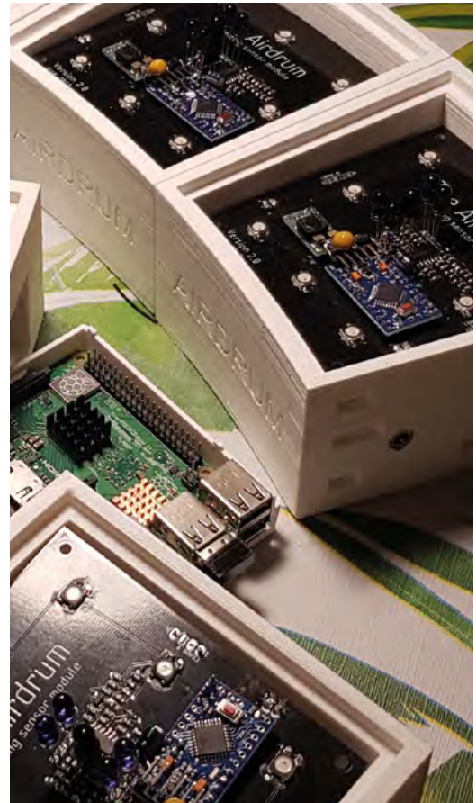
▶ Custom-made Airdrum detecting modules fit snugly into their 3D-printed cases and can be arranged in a full circle if you have enough of them
