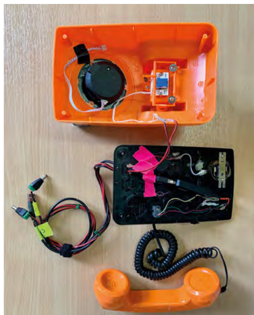
▲ Dave says it was easy to snip the wires from each phone's speaker, mic, and hang-up button and connect them to Raspberry Pi
