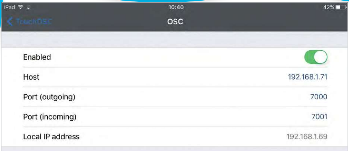
Fig 1: HOST: Set this to the address of the Raspberry Pi. Hover the pointer over the WiFi icon to find it.
