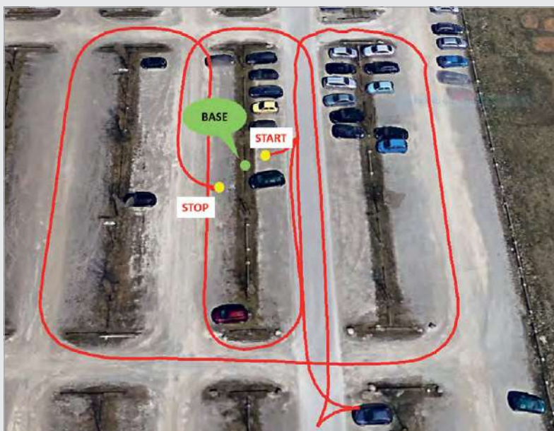
Left The path of a test drive, showing the precision of the system with a floating solution from the RTK calculation
