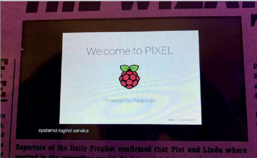
Above Both the glass of the frame and the bevel of the screen keep it fitted snugly within the newspaper, with no need for glue or screws
