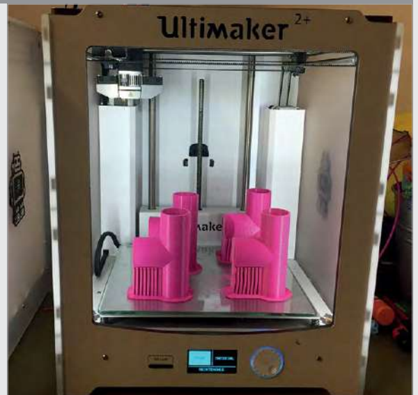
Above Eight cross joints and four T-junctions were 3D printed using an Ultimaker 2+
