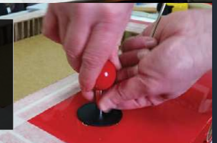
Holes drilled into the surface house the joystick and buttons. The controls are inserted from underneath
