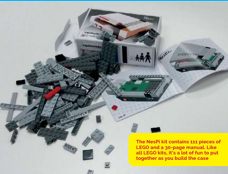
Putting the parts together results in this Raspberry Pi case. It looks like a classic NES console, but with access to the Raspberry Pi ports. The lid (used for cartridges in the original NES) provides access to the GPIO pins
