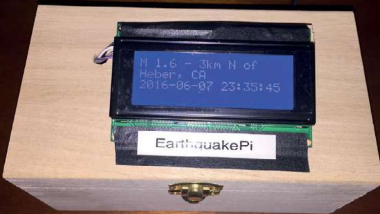
The Earthquake Pi – without optional NeoPixel bar graph – showing an alert for a small quake in California
