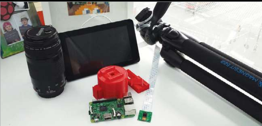
Above All the components James used for the project, including the red 3D printed lens adapter in three parts, which he later wrapped in duct tape
