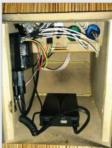
Above A hollowed-out interior houses the Raspberry Pi and the wires for the authentic arcade parts
