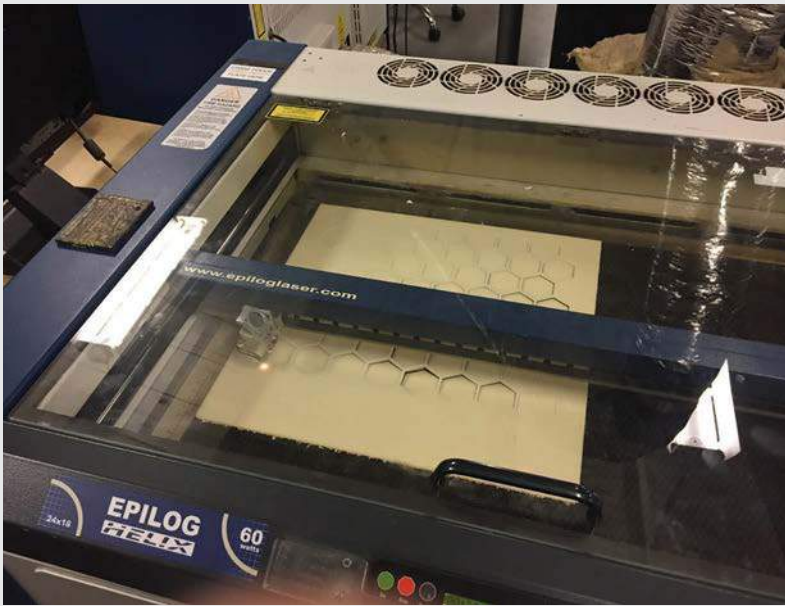
Above A laser cutter being used to cut the piece of acrylic.
