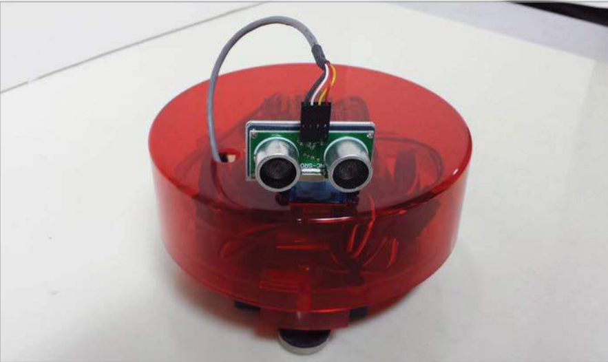
Above The finished product is a friendly-looking turtle-style robot that can sense objects in front of it
