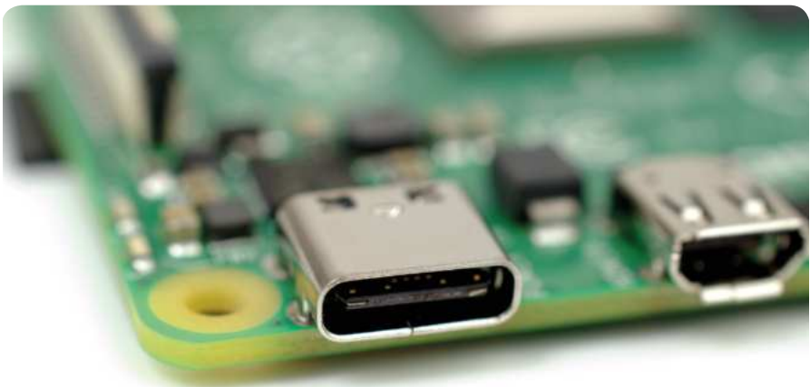
▲ Figure 1-11: The Raspberry Pi's USB Type-C power port
