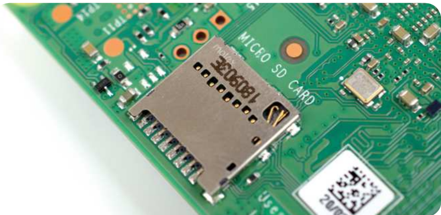
▲ Figure 1-15: The Raspberry Pi's microSD card connector
