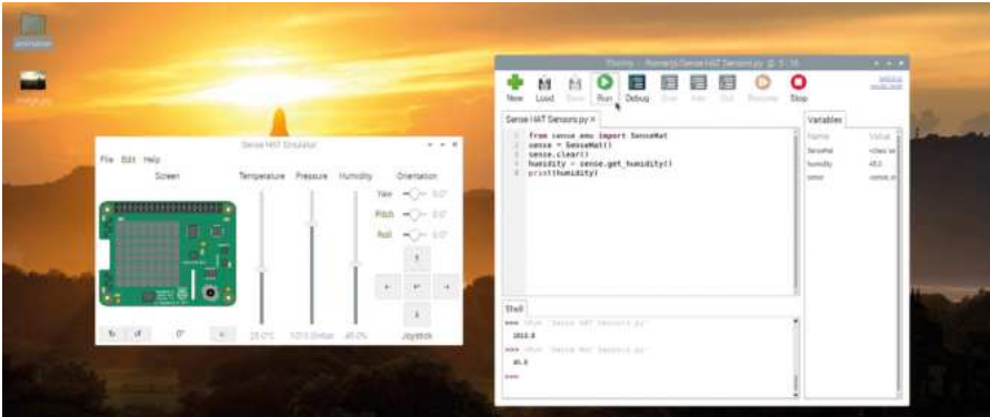
▲ Figure 7-22: Displaying the humidity sensor reading
