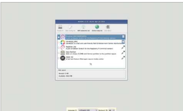
◀ Figure 2-1: The NOOBS menu without any operating systems installed
