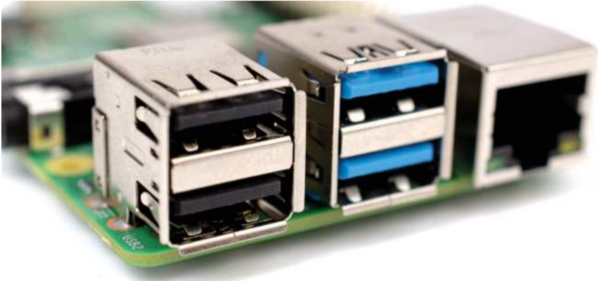
▲ Figure 1-6: The Raspberry Pi's USB ports
