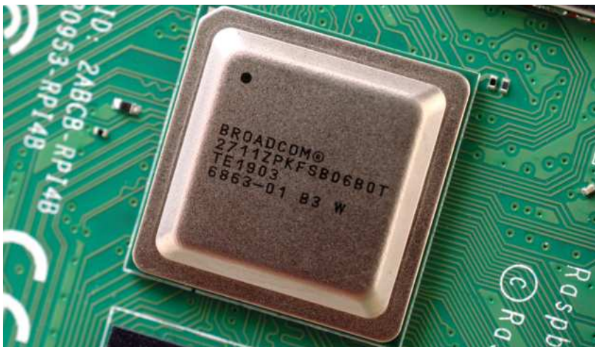
◀ Figure 1-2: The Raspberry Pi's system-on-chip (SoC)
