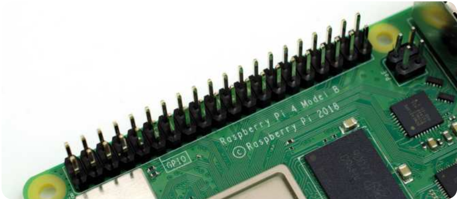
▲ Figure 1-14: The Raspberry Pi's GPIO header
