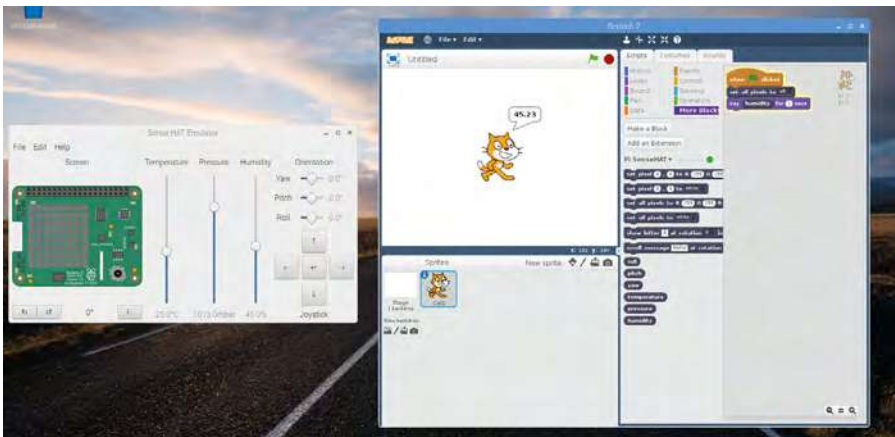
▲ Figure 7-19: Displaying the reading from the humidity sensor
