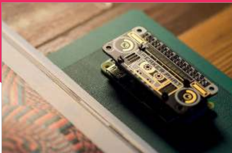
Right Use a speaker and microphone to turn your Pi Zero W into a hands-free Amazon Alexa Echo
