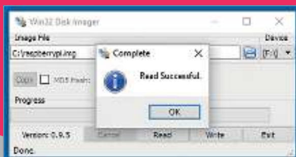
Above: You can clone your SD card to an image file using dd on a Mac or Linux, and Win32 Disk Imager on a PC
