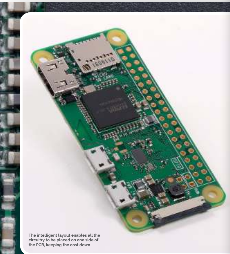
The white text is added to the PCB using a silk-screen technique. These markings are used to provide information and branding for the board
