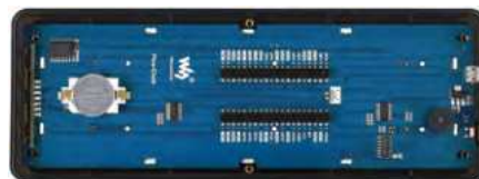
▲ A Raspberry Pi Pico flashed with the software can be slotted into the clock's rear female headers
