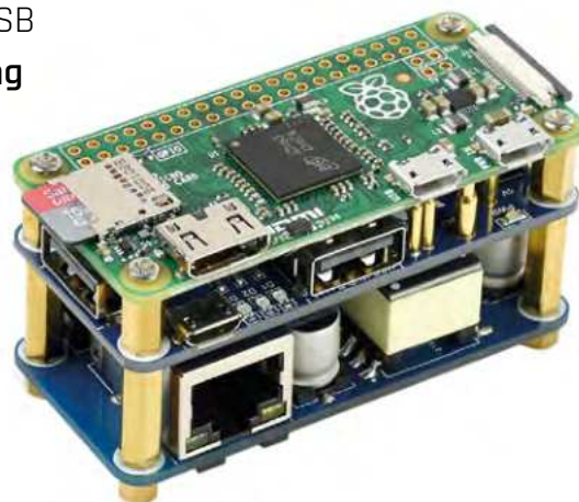
▲ With Raspberry Pi Zero mounted on top, the double-decker HAT adds three USB ports on the top board and PoE on the bottom
