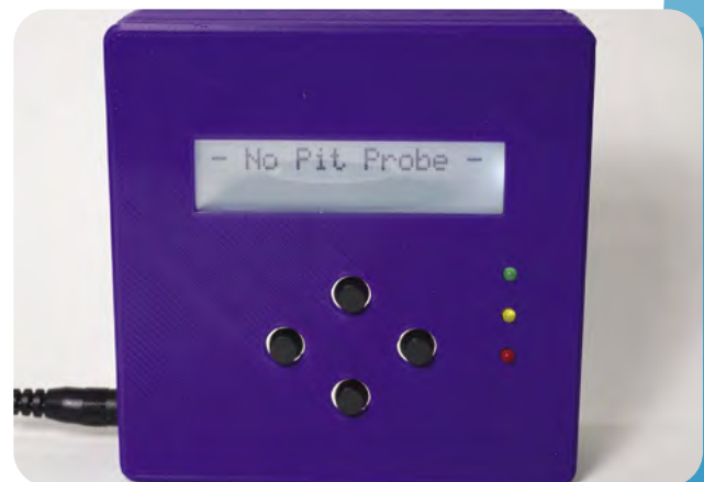
▼ HeaterMeter lets you keep an eye on your BBQ from a distance, freeing you to get on with prep in the kitchen while the HeaterMeter maintains cooking temperatures
