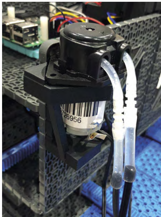
◀ A pump is used to supply water to the system
