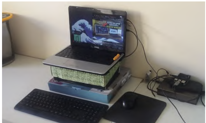
▼ Rafa used an old notebook as a screen for a desktop Raspberry Pi setup
