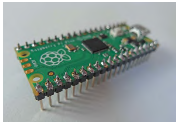
▲ With the USB socket uppermost, the longer legs on your soldered headers should point downwards
