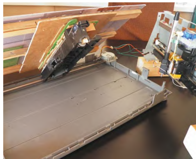
▶ Lifting up the drawing surface reveals the old scanner parts below, as well as the platform’s stepper motor
