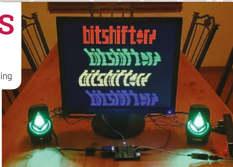
▲ The BBC Micro computer emulated on Raspberry Pi Pico, with PIO handling the display output
