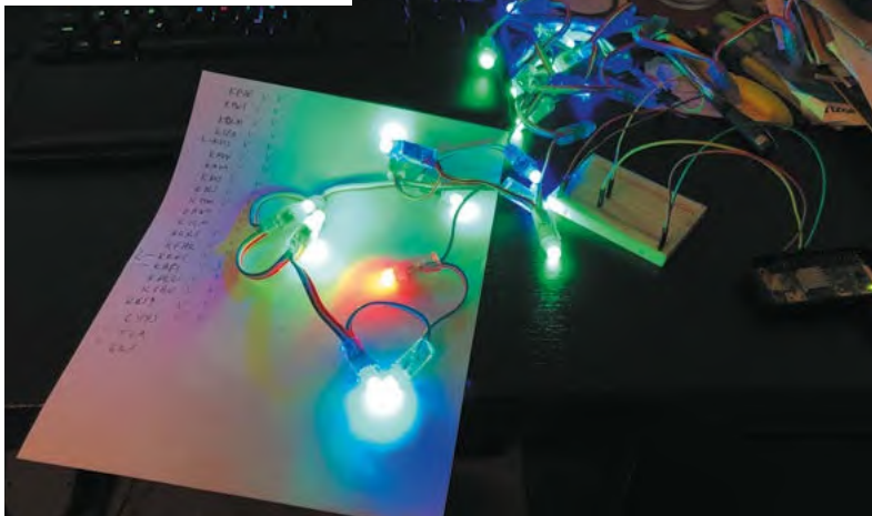
▼ Testing the code on a string of LEDs before taping them to back of the map
