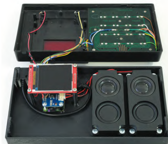
▲ The inner workings include a Raspberry Pi Zero with WM8g60 Audio HAT, speakers, and 176x220 LCD
