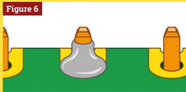
▲ Figure 6 A well-soldered pin
