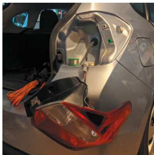
▲ A voltage divider and signal wire to the reverse lamp circuit in the rear light connect to a GPIO pin on Raspberry Pi. The reversing camera is summoned whenever the car is put into reverse
