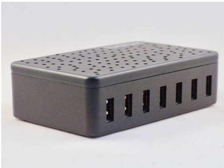
▲ Instead of a row of wall-warts, use a multi-port USB charger to power your cluster nodes, but make sure your choice of unit has enough amps
