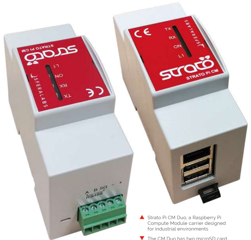
▼ The CM Duo has two microSD card slots, creating a platform that can be updated while still running
