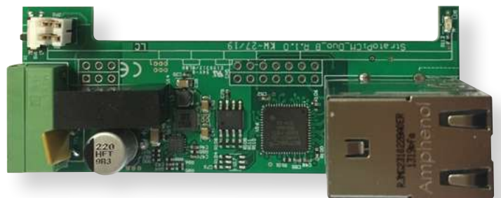
▼ The CM Duo has two microSD card slots, creating a platform that can be updated while still running
