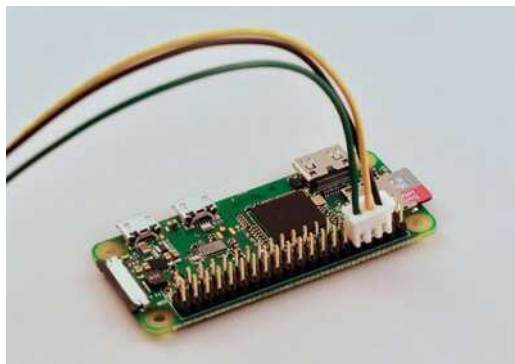
▲ Luckily, the printer's connector matches up with the GPIO pins and can be directly attached
