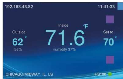
▲ Viewable via VNC on a smartphone, the program window features temperature data and control buttons
