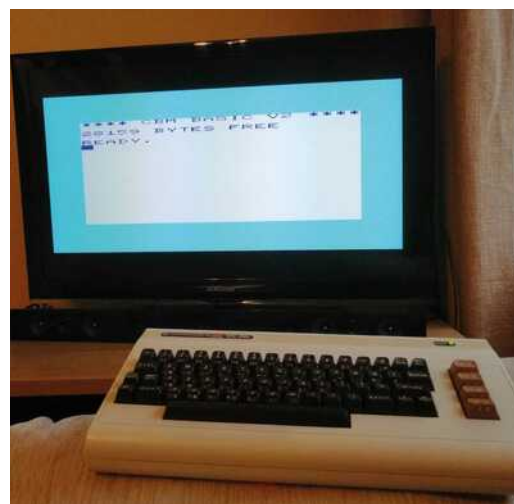
▲ When PIC-20 is connected to a monitor, it looks and behaves like an original VIC-20 from the 1980s
