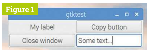
▲ Figure 1 A GtkEntry added to the bottom-right of the table
