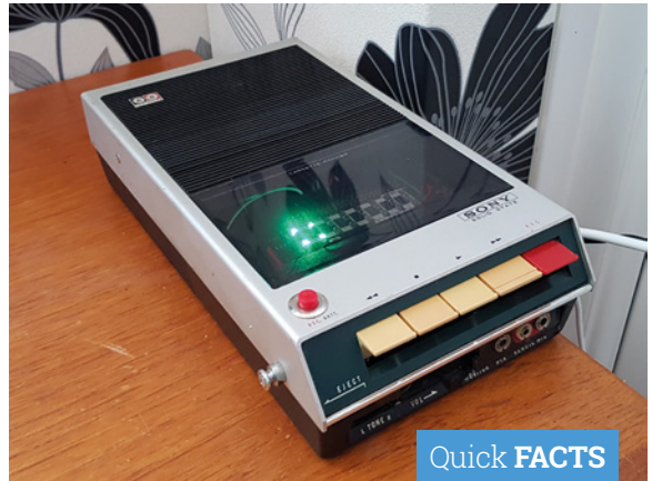
▲ Raspberry Pi and PHAT BEAT are placed inside an old cassette player wired to the intercom outside. The PHAT BEAT is also connected to the player's original speaker so that speech and the chime can be heard
