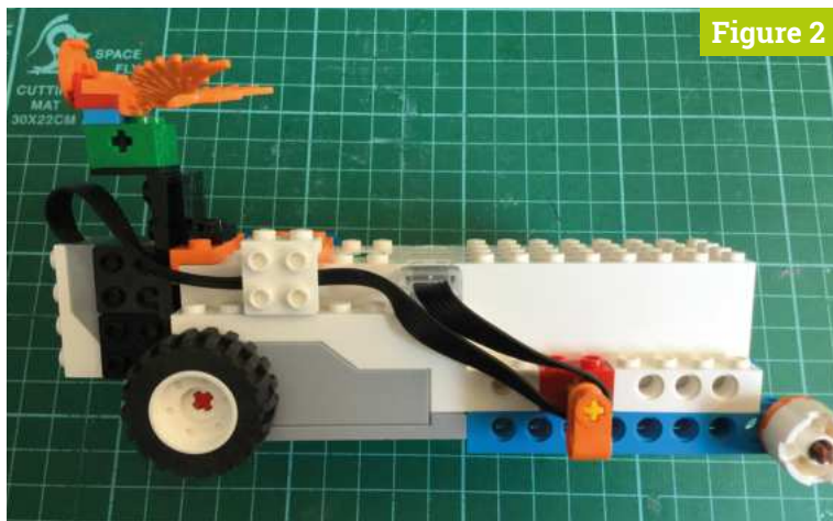
▲ Figure 2 How to tidy up the colour sensor's wire
