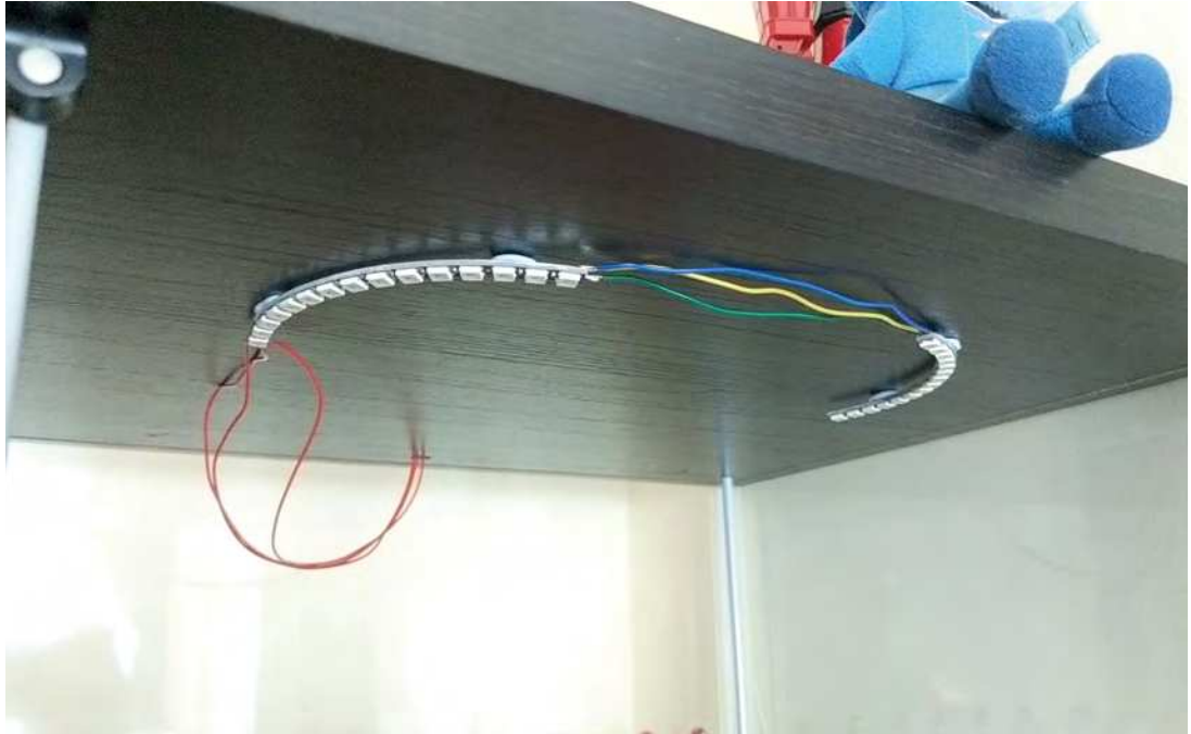
► We used Blu Tack to attach the lights to the top of our cabinet
