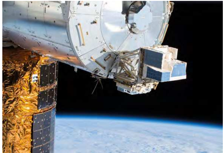
▲ The ARISS VHF antenna installed on the bottom of the Columbus module Credit: NASA/ESA
