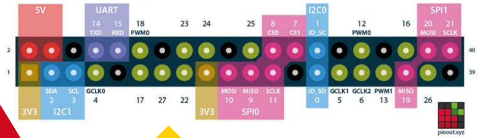
Raspberry Pi GPIO BCM numbering
