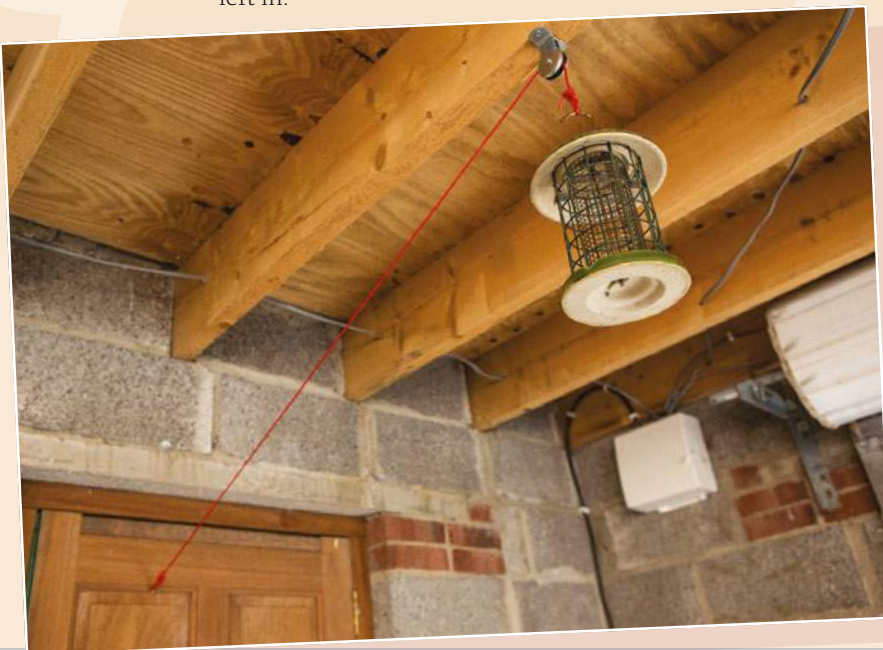
Left The door is connected to a weight via a pulley system. When the actuator moves back, the door automatically swings open
