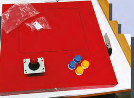
A square in the table is cut to contain the 17-inch display. The wood is then prised out to reveal the structural filling inside
