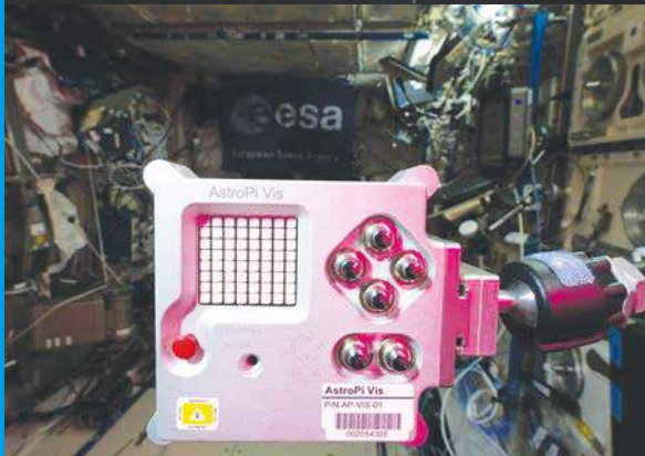
Above The Sense HAT and Raspberry Pi module, to be used by Tim Peake to perform Astro Pi experiments aboard the ISS
