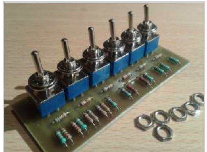
The switches are placed on the circuit board, but not soldered yet.
