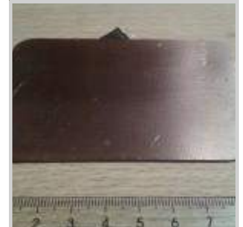
The base, made of copper clad.
