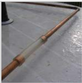
A piece of not-too-flexible PVC tube is used to fix the end points of the dipole.
