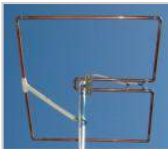
Bill VE3BXP is one of the many radio amateurs who built this antenna, inspired by this article on my website. He added an extra support by using a PVC pipe and T-junction, which also acts as an insulator.
