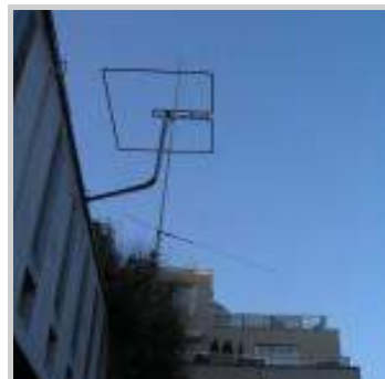
The squalo on its definitive place, next to the Diamond 6/2/70 vertical, on the balcony rail on the south side of Adri's apartment.
