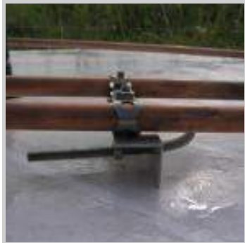
The mount bracket. I used a aluminium strip for this, but you better use some more solid metal for this.
