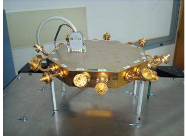
NIST researchers developed this directional 16-antenna array to support modeling of wireless communications channels at 83 gigahertz.
