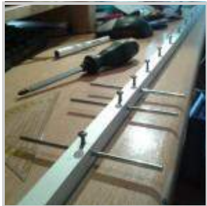
Placing the elements, be sure to center them for the best result.
