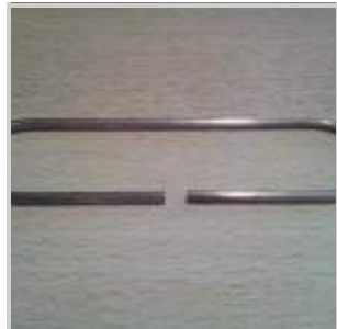
The copper dipole, I bended this using a metal pipe.
