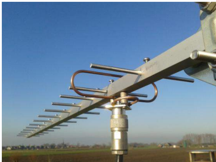
My 23cm Yagi antenna, in fixed position to the local ATV repeater.
