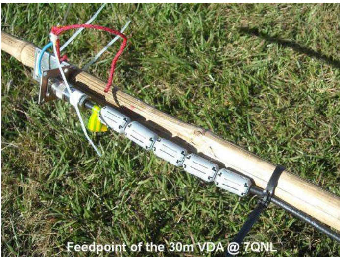
Picture 12 Feedpoint of the 7QNL 30m VDA using five 2 \mu\text{H} ferrite clamps as common mode choke.
