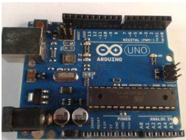
The Arduino prototype board, this is the "Uno" version. Throughout the years several versions have been released, but all are code and pin compatible.
