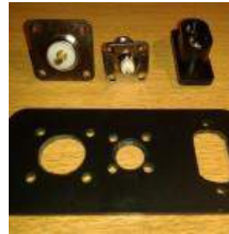
Cutting and drilling the holes for the connectors, switch and LED fitting always takes some time. Good measurement and a drill press ensure a nice result.
