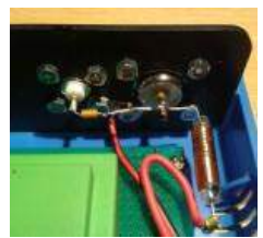
Detail of the RF part. Notice the small cap between the 2 connectors, that will block all DC. The large inductor blocks the RF while passing by the DC cur-
