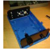
After all cutting and drilling is done, the connectors, switch and LED can be mounted. Notice the metal strip between the RF connectors to connect the chassis.
